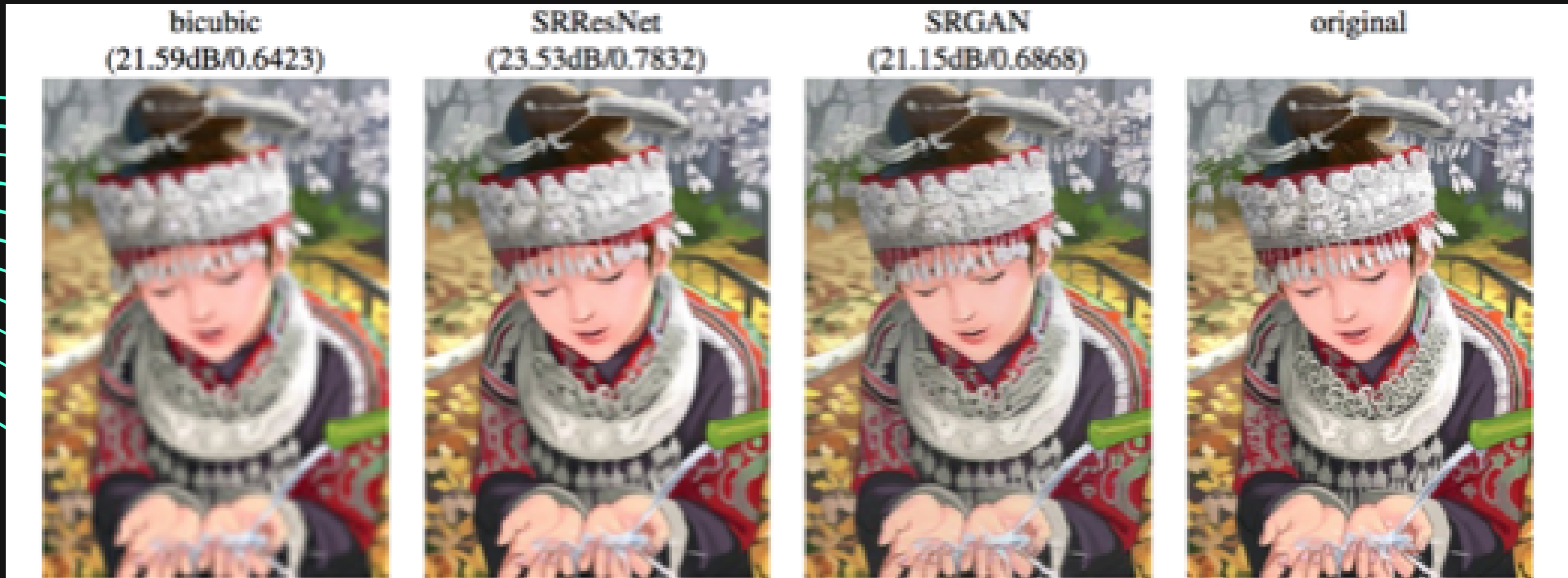
Figure 2: From left to right: bicubic interpolation, deep residual network optimized for MSE, deep residual generative adversarial network optimized for a loss more sensitive to human perception, original HR image. Corresponding PSNR and SSIM are shown in brackets. [4x upscaling]
