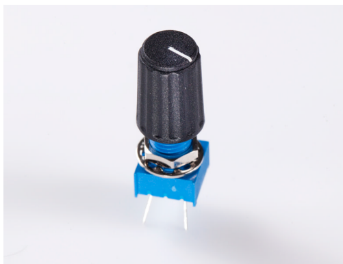
Figure 3-10. Potentiometers can measure rotation
