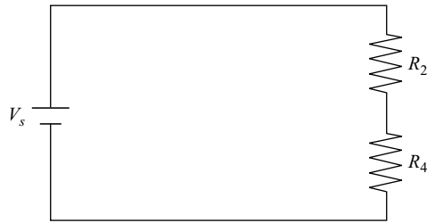
Fig. 3-20 The two resistors on the right-hand edge of Fig. 3-19 are in series.
